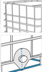
**4. Cutout Width at Outlet Valve:** Cutout Width at Outlet Valve of the IBC Tote
